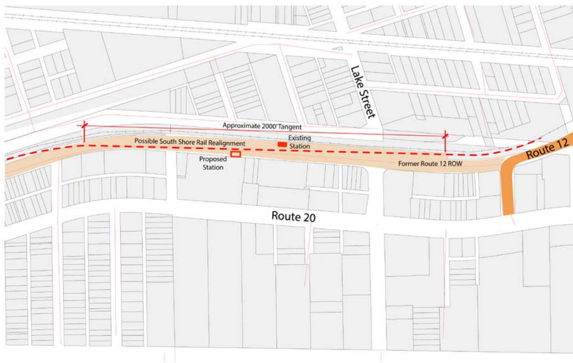
Figure 10: Strategy to Realign the Rail in the Vacated Route 12 Right of Way
