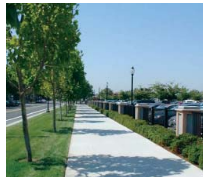
Screen the edges of parking lots that face onto a street with trees and other plantings.
